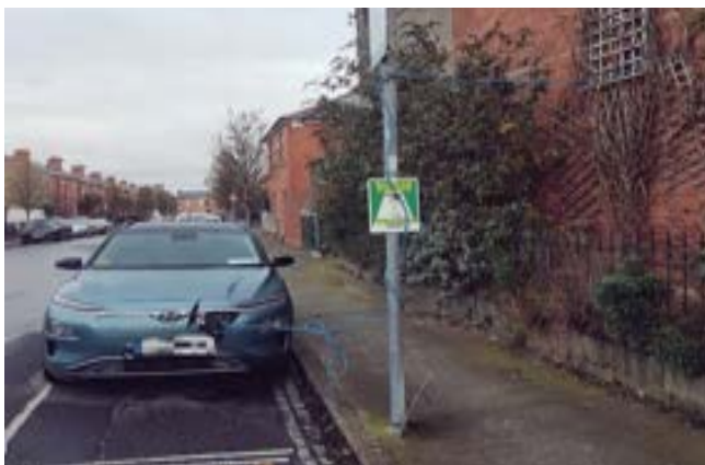
Figure 14: EV charging cable running from private residence to Traffic sign to EV in Dublin (Source: Twitter)
