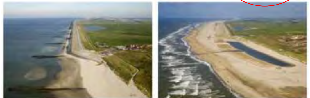
Figure 2a and 2b. (below) Illustration of "hard" versus "soft" engineering. The photo on the left shows the original "Hondsbossche en Pettemer Zeewering", a large dike in North Holland, whereas the photo on the right shows the same construction fortified by sand nourishment rather than additional hard structures. (Photo credit: Boskalis.)
