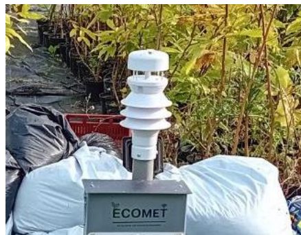
Figure 3. Ecomet tool (mini weather station tool) for metrological parameters measurement, including air temperature, relative humidity, precipitation (radar based), water vapor pressure, air pressure, wind speed and wind direction.
